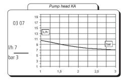
Flow rate indicated is for  $H_2$ O at 20°C at the rated pressure. Dosing accuracy  $\pm$  2% at constant pressure  $\pm$  0,5 bar.
