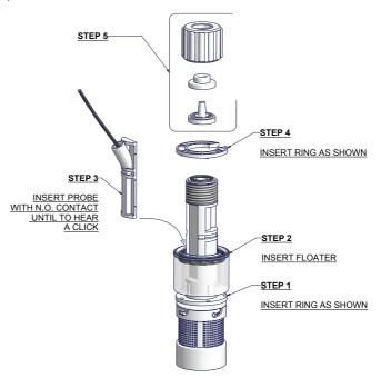
Connect BNC from level probe into pump's level input (front side of the pump). Put level probe assembled with foot filter into tank's bottom.
