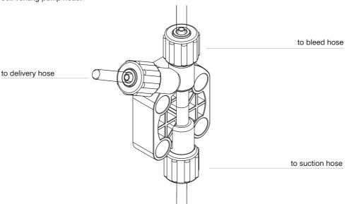
Self-venting pump head must be used when using chemicals that produce gas (i.e. hydrogen peroxide, ammonium, sodium hypoclorite at particular conditions).
