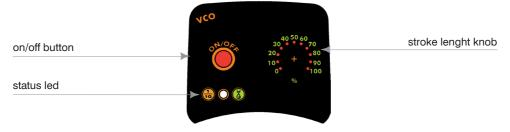
LED The led on the frontal panel shows the pump's operating status through 5 flashing:
