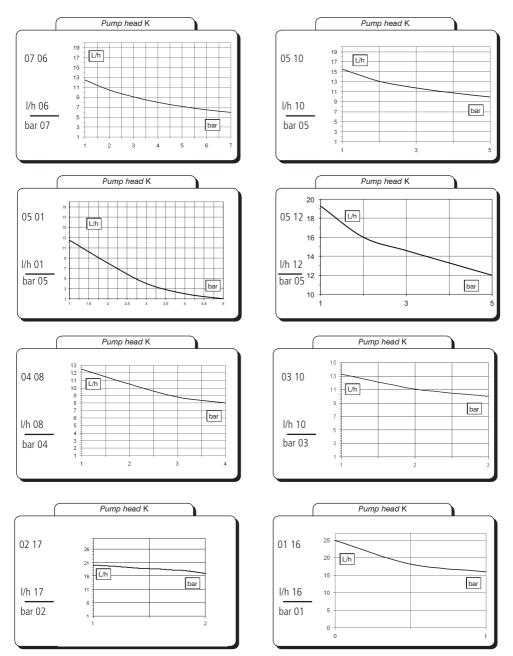
Flow rate indicated is for  $H_2O$  at  $20^{\circ}C$  at the rated pressure. Dosing accuracy  $\pm$  2% at constant pressure  $\pm$  0,5 bar.
